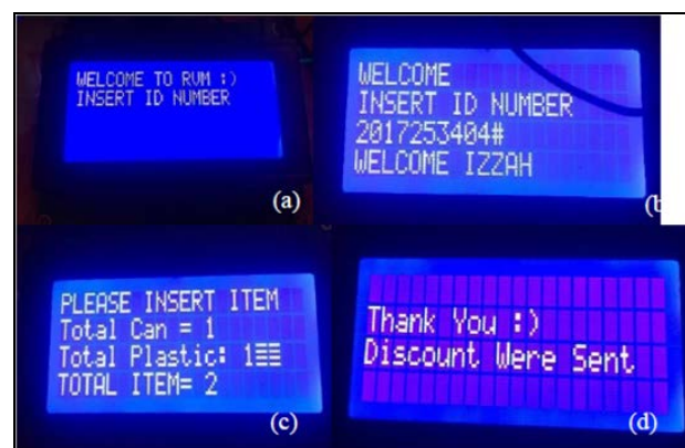
Fig 6: LCD display for (a) prompting user to enter ID number, (b) displaying registered user ID and name, (c) showing the number and type of items inserted by the user, (d) displaying appreciation and discount confirmation to the user.
