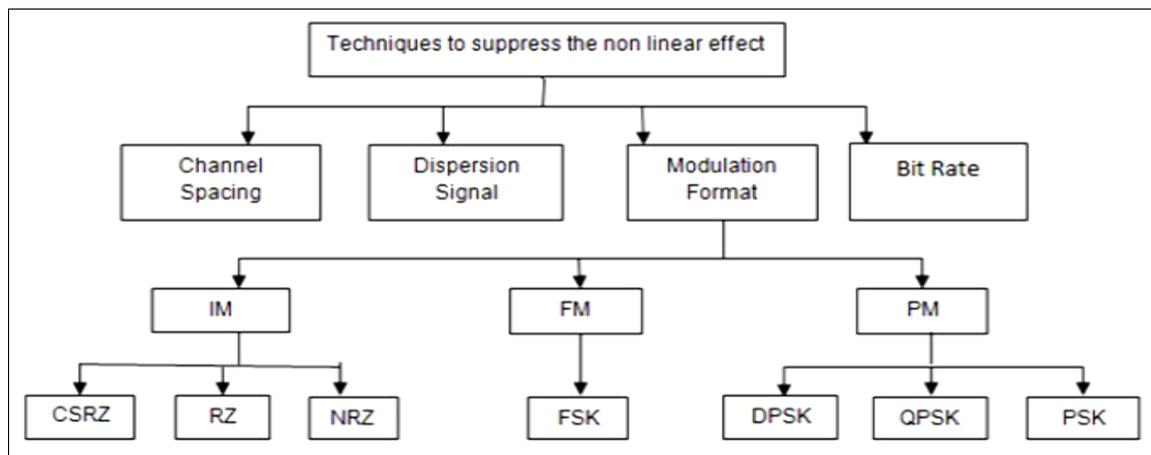
Fig 5: Classification of Modulation Formats
