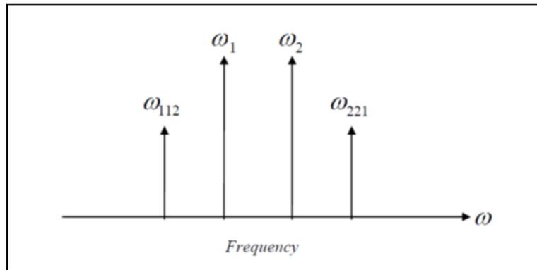
**Fig 4:** Additional frequencies generated through FWM.
