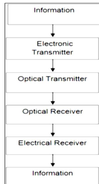
Fig.1: Communication System of Fiber-Optic
