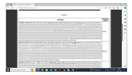
The first column of the screen above shows test data from user behaviour; the second column shows the transaction status as either normal or fraudulent.
