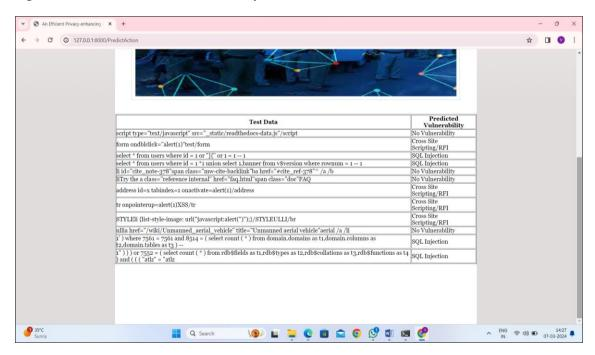
Predicted vulnerabilities are shown in the second column of the table, whereas SQL queries, XSS, and RFI coding instructions are shown in the first column.
