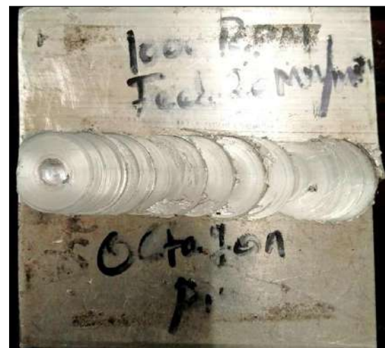
Fig 3.8: Weld at 1000 rpm, feed 20 mm/min, and depth 5.6 mm
