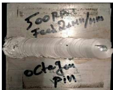
Fig 3.7: Weld at 500 rpm, feed of 20 mm/min and depth is 5.6 mm The trial welding was conducted on AA2024 and AA6061 with octagonal pin with parameters 700 rpm with feed of 20 mm / min and depth was given as 5.6 mm. the result obtained was a onion rings with a small crack due to excessive temperature distribution and pilot hole was formed at the end.
