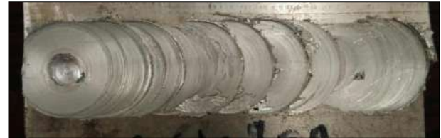
Fig 4.3: Good weld with crack obtained at starting stage due to temperature distribution in 1000 rpm rotational speed, transvers speed 20 mm/min
