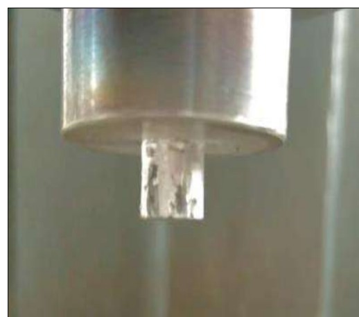
Fig 3.9: after weld of pin at 710 rpm
