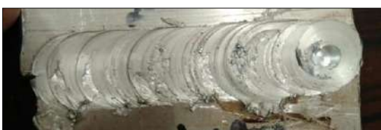
Fig 4.2: Defect weld due to improper weld obtained at 700 rpm transvers speed 20 mm/mm
