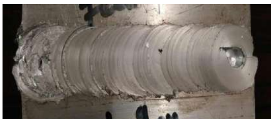
Fig 4.1: obtained defect at starting stage due to temperature distribution at 500 rpm, transvers speed 20 mm/min
