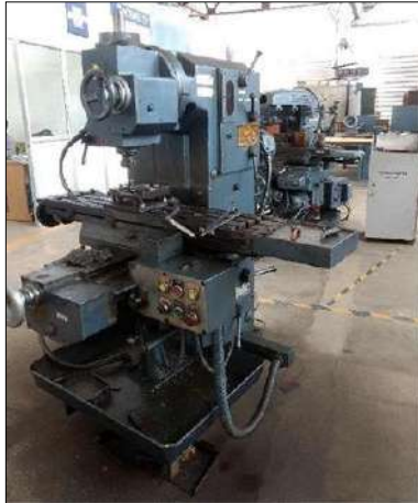
Fig 3.6: Retro Fixed Vertical Milling Machine
