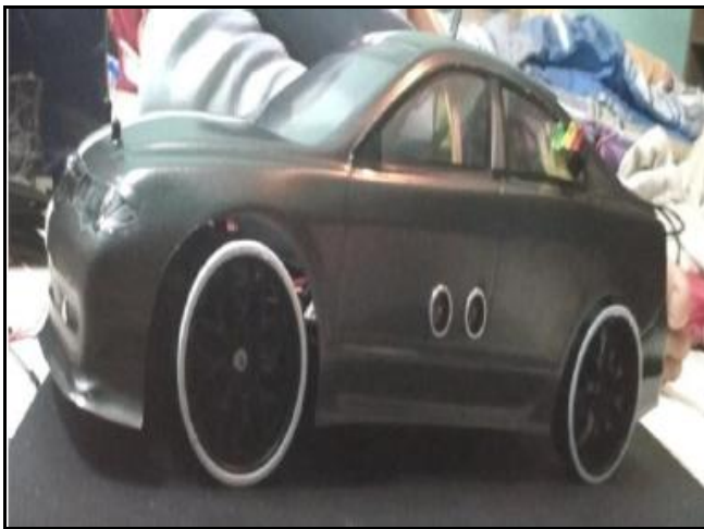
Fig 4: Remote control car prototype with Vehicle's Blind Spot Detector
