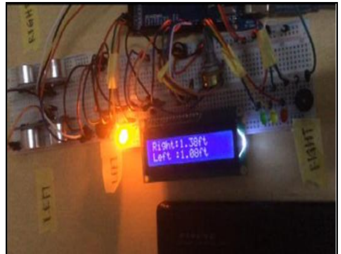
Fig 6: Sensor detects object between 1 feet to 2 feet distance
