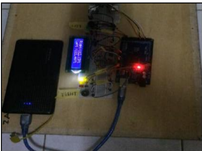
Fig 5: No object within 3 feet distance
