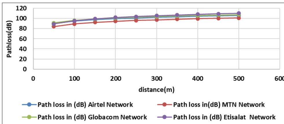
**Fig 2:** Measured path losses from the proposed modified for oke oniti
