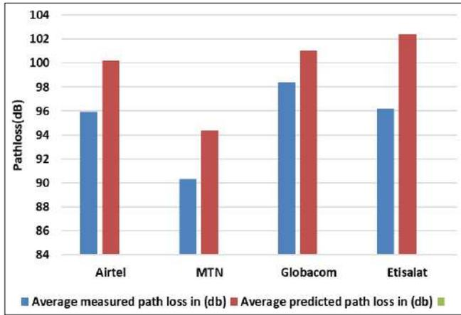
Fig 7: Measured and Predicted path losses for Odiolowo
